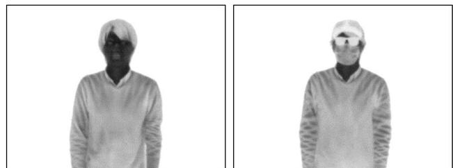
Fig. 2: Examples of images in thermal infrared spectrum. Left: An image of a person without a headgear. Right: An image of a person with headgears (hat, glasses, and mask).
