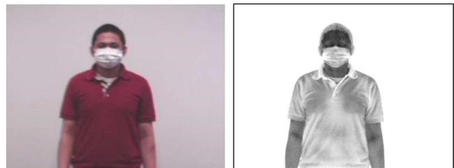
Fig. 1: Examples of images captured by cameras in different spectra. Left: An image captured in the visible spectrum. Right: An image captured in the thermal infrared spectrum.
